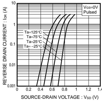
Fig.5 Reverse Drain Current vs. Source-Drain Voltage ( I )
