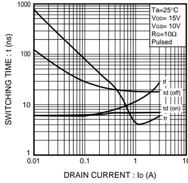
Fig.2 Switching Characteristics
