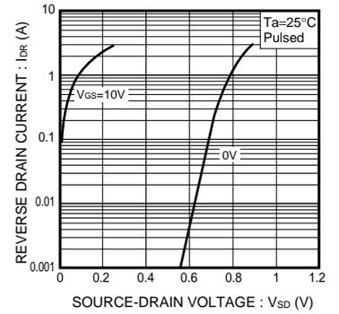
Fig.6 Reverse Drain Current vs. Source-Drain Voltage ( II )
