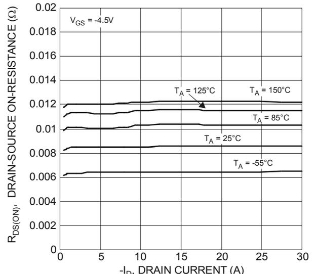
Figure 4 Typical On-Resistance vs. Drain Current and Temperature
