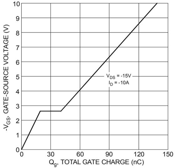
Figure 10 Gate-Source Voltage vs. Total Gate Charge
