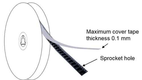
Figure 22. Reel dimensions (mm)
