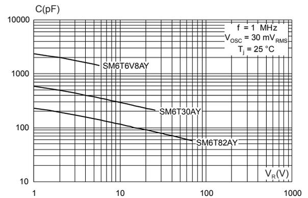
Figure 8. Junction capacitance versus applied voltage (bidirectional type)
