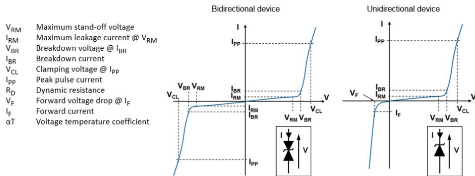
**Figure 3. Pulse definition for electrical characteristics**
