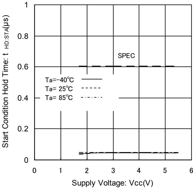
Figure 16. Start Condition Hold Time vs Supply Voltage
