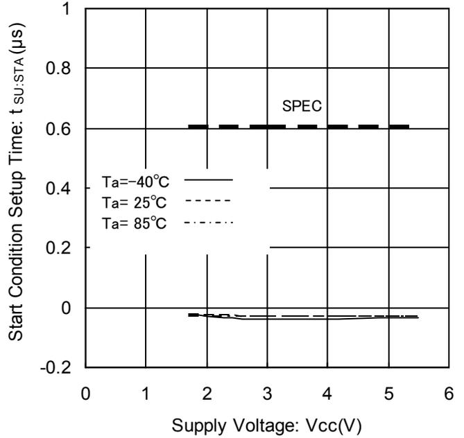
Figure 17. Start Condition Setup Time vs Supply Voltage
