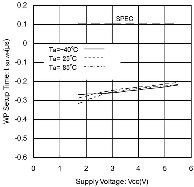
Figure 32. WP Setup Time vs Supply Voltage
