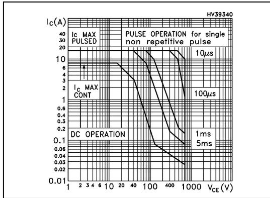
Figure 3. Derating curve
