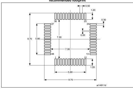
Figure 63. LQFP48 - 48-pin, 7 x 7 mm low-profile quad flat package recommended footprint
