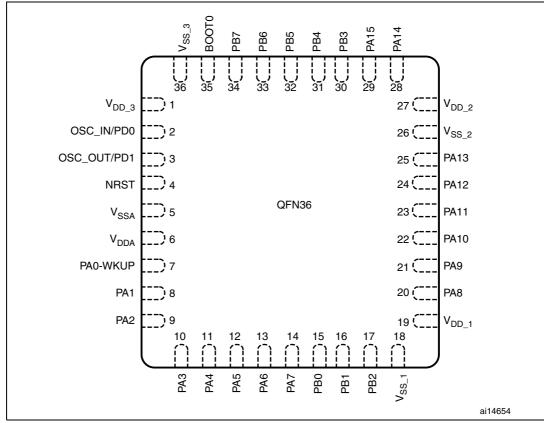
Figure 10. STM32F103xx performance line VFQFPN36 pinout
