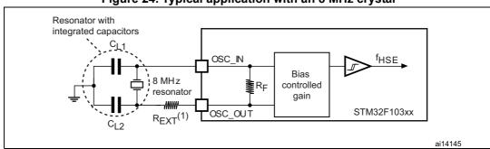
Figure 24. Typical application with an 8 MHz crystal
