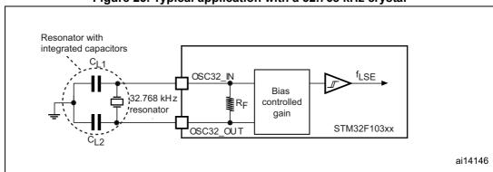
Figure 25. Typical application with a 32.768 kHz crystal
