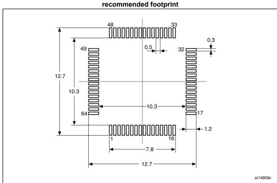
Figure 57. LQFP64 - 64-pin, 10 x 10 mm low-profile quad flat package recommended footprint
