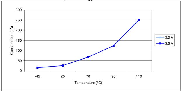
Figure 20. Typical current consumption in Stop mode with regulator in Low-power mode versus temperature at  $V_{DD}$  = 3.3 V and 3.6 V
