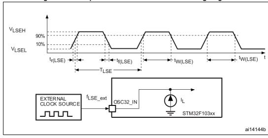
Figure 23. Low-speed external clock source AC timing diagram
