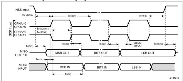
Figure 33. SPI timing diagram - slave mode and CPHA = 0
