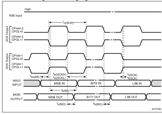
Figure 35. SPI timing diagram - master mode<sup>(1)</sup>
