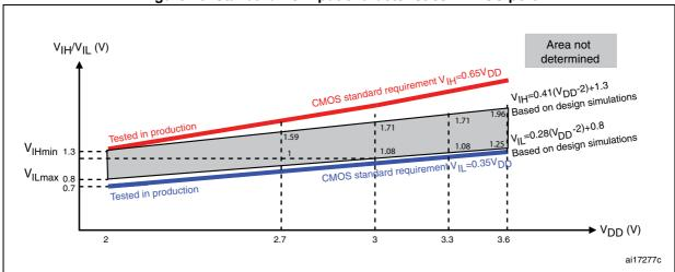
Figure 26. Standard I/O input characteristics - CMOS port
