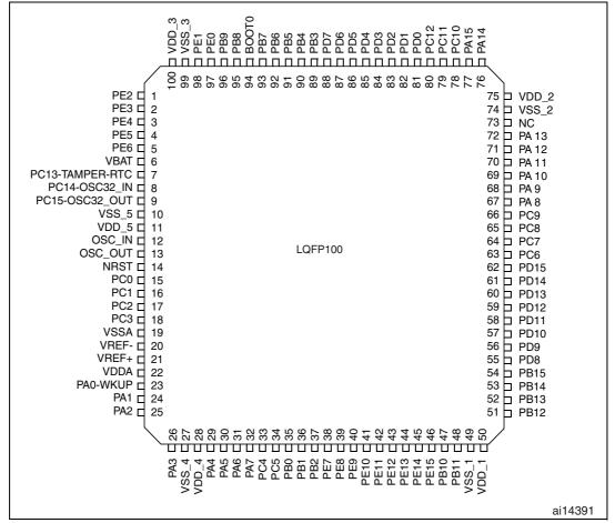
Figure 4. STM32F103xx performance line LQFP100 pinout
