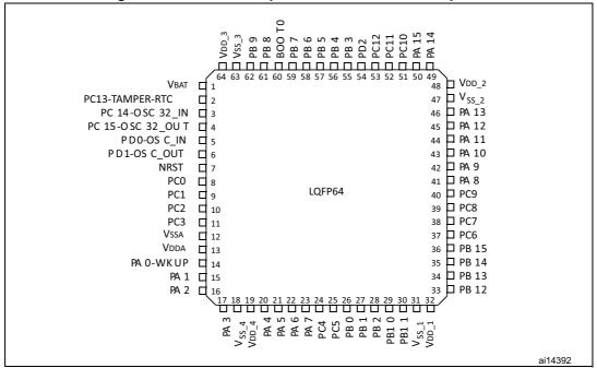
Figure 6. STM32F103xx performance line LQFP64 pinout
