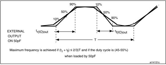
Figure 30. I/O AC characteristics definition
