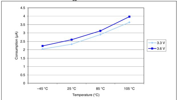
Figure 21. Typical current consumption in Standby mode versus temperature at  $V_{DD}$  = 3.3 V and 3.6 V
