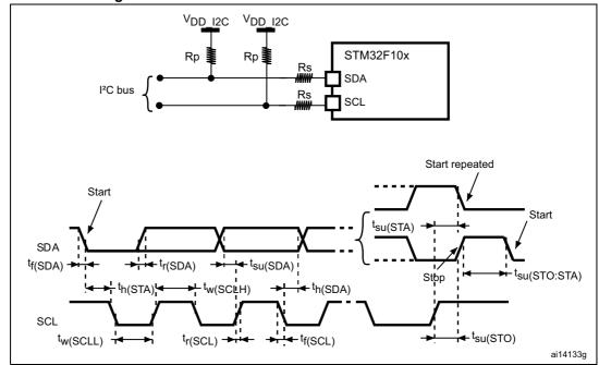
Figure 32. I<sup>2</sup>C bus AC waveforms and measurement circuit
