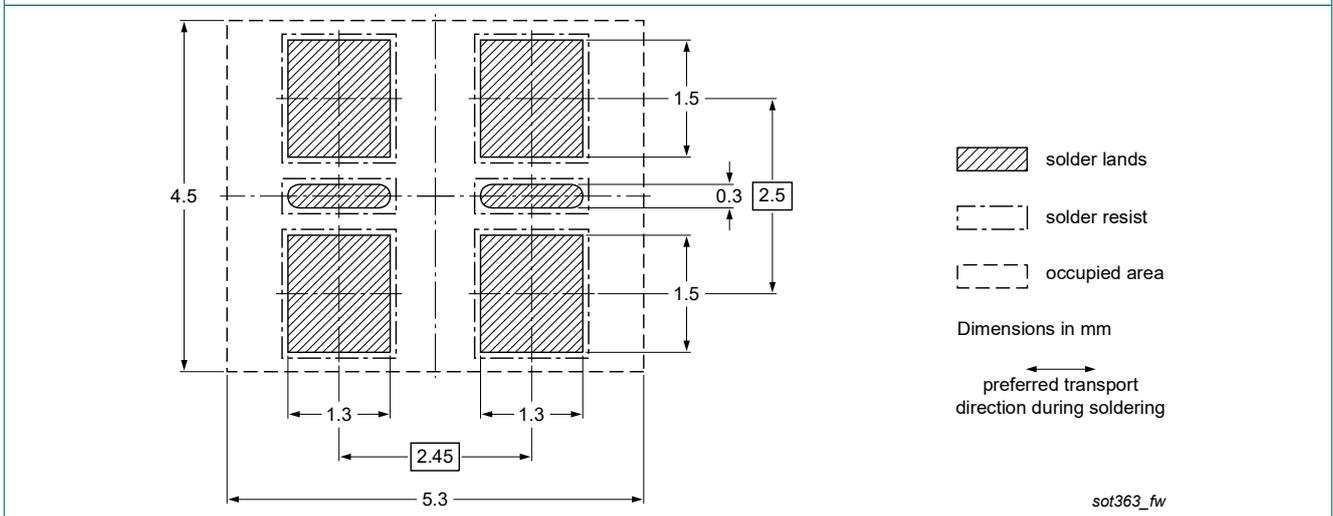
Fig. 11. Wave soldering footprint for TSSOP6 (SOT363)
