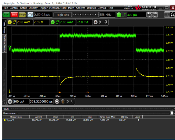
Figure 13. Load Transient, \pm 2 mA, V_{IN} = 5 V, C_{IN} = 1 \mu F, C_{OUT} = 1 \mu F, 20 mV/div
