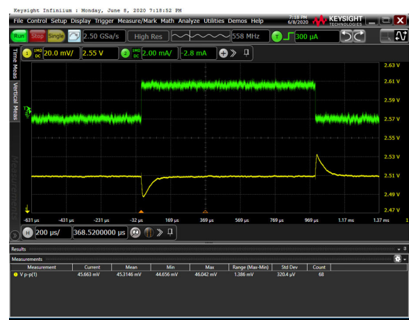
Figure 14. Load Transient, \pm 2 mA, V_{IN} = 2.8 V, C_{IN} = 1 \mu F, C_{OUT} = 1 \mu F, 20 mV/div
