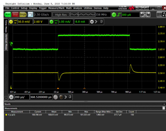
Figure 12. Load Transient, \pm 5\text{ mA} , V_{IN} = 2.8\text{ V} , C_{IN} = 1\text{ }\mu\text{F} , C_{OUT} = 1\text{ }\mu\text{F} , 50 mV/div
