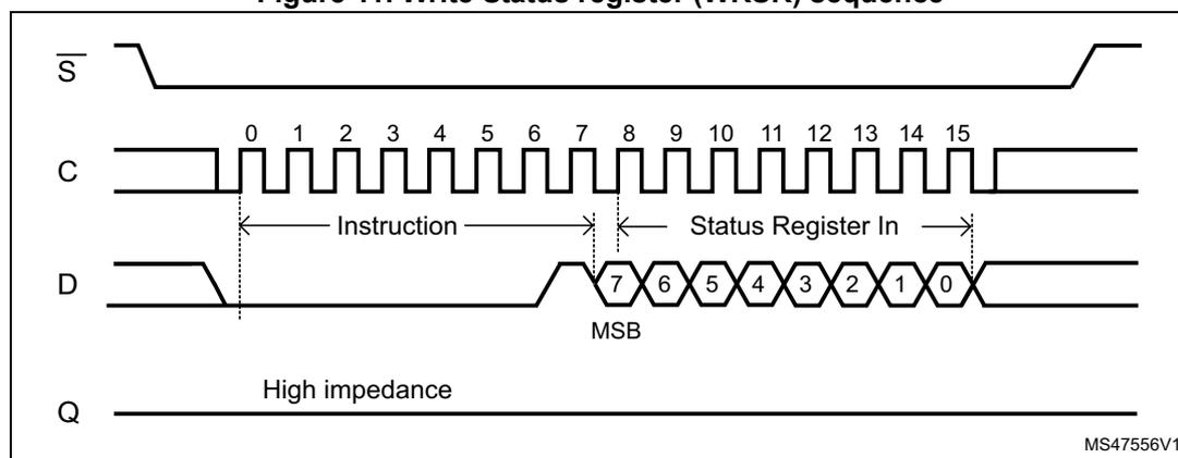
Driving the Chip select ( $\bar{S}$ ) signal high at a byte boundary of the input data triggers the self-timed Write cycle that takes  $t_{\text{W}}$  to complete (as specified in AC tables in [Section 9: DC and AC parameters](#)).
