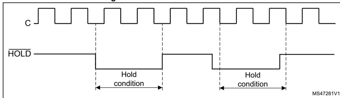
The Hold condition starts when the Hold ( $\overline{HOLD}$ ) signal is driven low when Serial clock (C) is already low (as shown in [Figure 7](#)).
