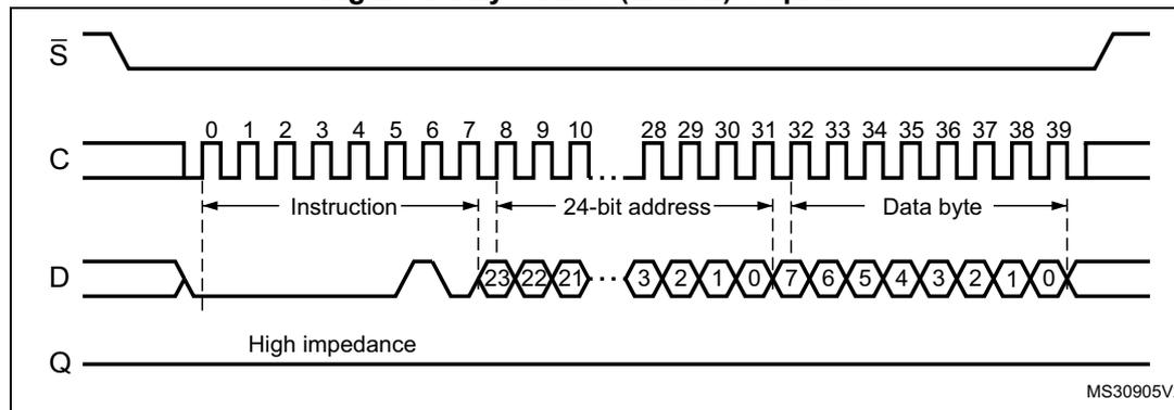
In the case of [Figure 13](#), Chip select ( $\bar{S}$ ) is driven high after the eighth bit of the data byte has been latched in, indicating that the instruction is being used to write a single byte. However, if Chip select ( $\bar{S}$ ) continues to be driven low (as shown in [Figure 14](#)), the next byte of input data is shifted in, so that more than a single byte, starting from the given address towards the end of the same page, can be written in a single internal Write cycle.
