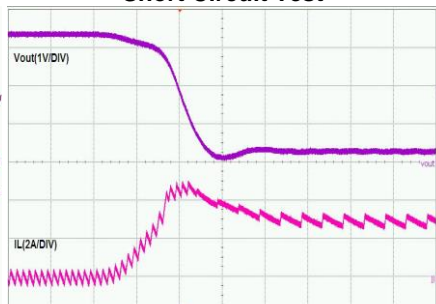
Short Circuit Test
