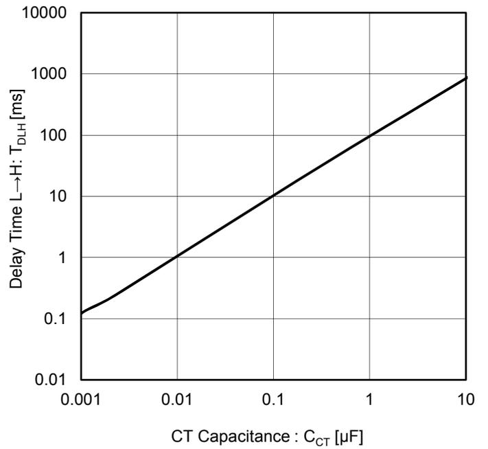
Figure 14. Delay Time L→H vs. CT Capacitance
