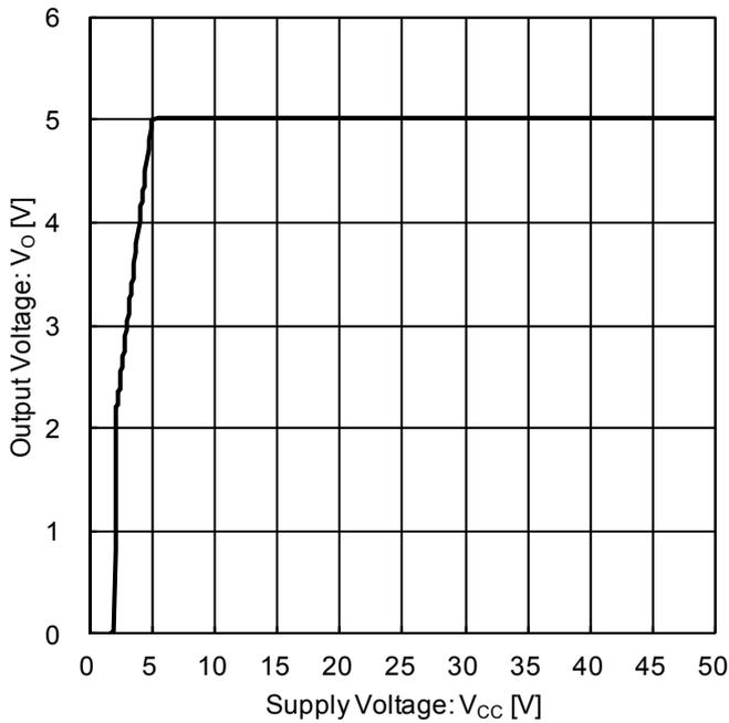
Figure 1. Output Voltage vs. Supply Voltage ( $R_L = \text{open}$ )
