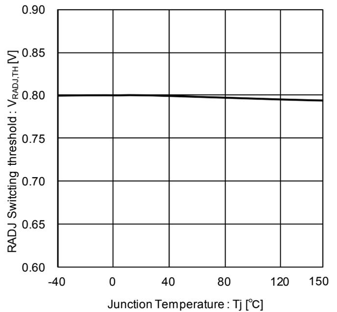
Figure 16. RADJ switching threshold vs. Junction Temperature
