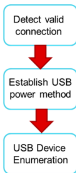
图 11. Flow of DFP to UFP Configuration
