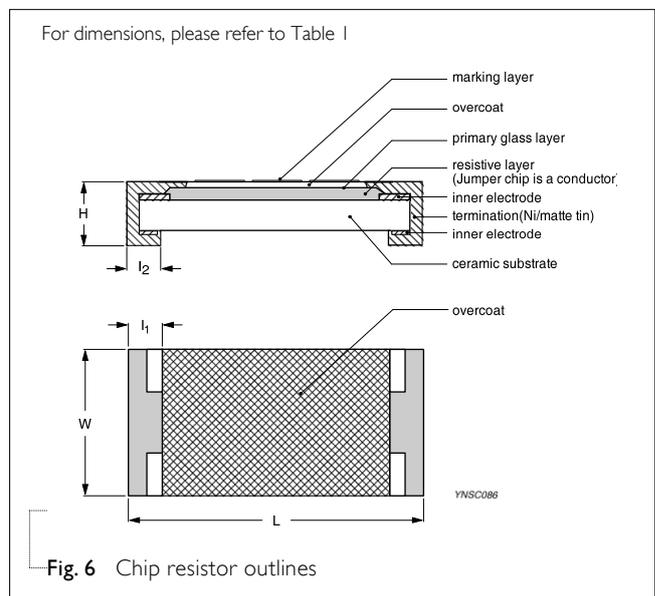
Fig. 6 Chip resistor outlines
