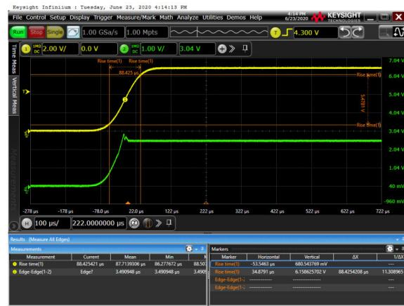
Figure 7. Power up, 100  $\mu\text{s}$ ,  $V_{BIAS} = 6.5 \text{ V}$ ,  $R_{BIAS} = 2.5 \text{ k}\Omega$
