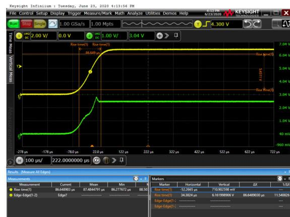
Figure 9. Power up, 100  $\mu\text{s}$ ,  $V_{BIAS} = 6.5 \text{ V}$ ,  $R_{BIAS} = 20 \text{ k}\Omega$
