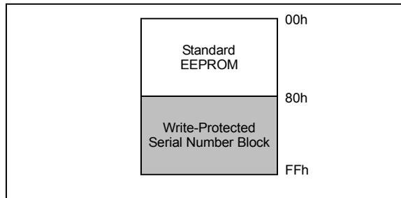
The 4-byte serial number is stored in array locations 0xFC through 0xFF, as shown in Figure 9-2.
