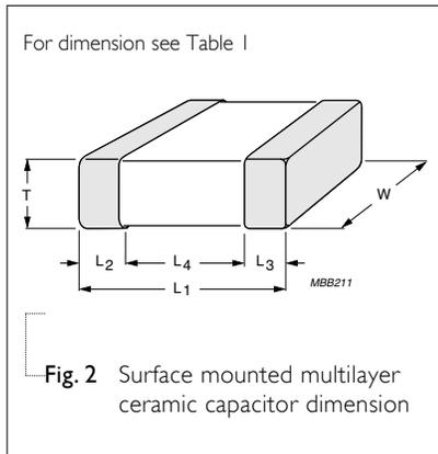
Fig. 2 Surface mounted multilayer ceramic capacitor dimension
