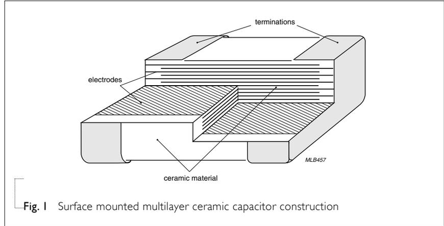
Fig. 1 Surface mounted multilayer ceramic capacitor construction
