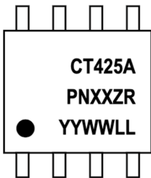
Figure 45: CT425 Device Marking for 8-lead Package
