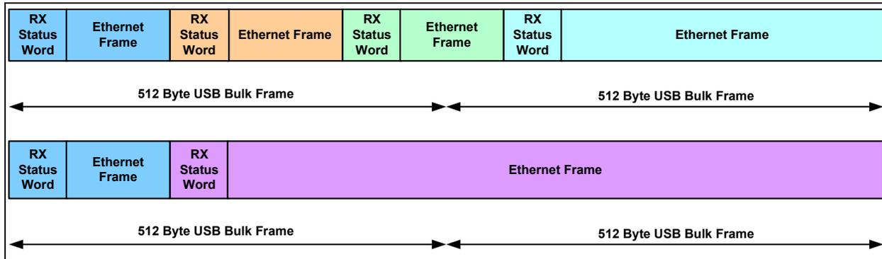
In accordance with the USB protocol, the UTX terminates a burst with either a ZLP or a Bulk-In packet with a size of less than the Bulk-In maximum packet size (512 bytes). The ZLP is needed when the total amount of data transmitted is a multiple of a Bulk-In packet size. The UTX monitors the RX FIFO size signal from the FCT to determine when a burst has ended.
