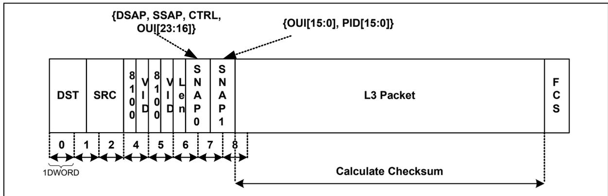
The RXCOE supports a maximum of two VLAN tags. If there are more than two VLAN tags, the VLAN protocol identifier for the third tag is treated as an Ethernet type field. The checksum calculation will begin immediately after the type field.
