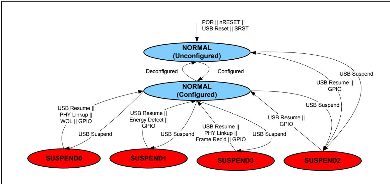
**Note:** It is not possible to transition from SUSPEND2 to NORMAL Configured if SUSPEND2 was entered via a transition from NORMAL Unconfigured.
