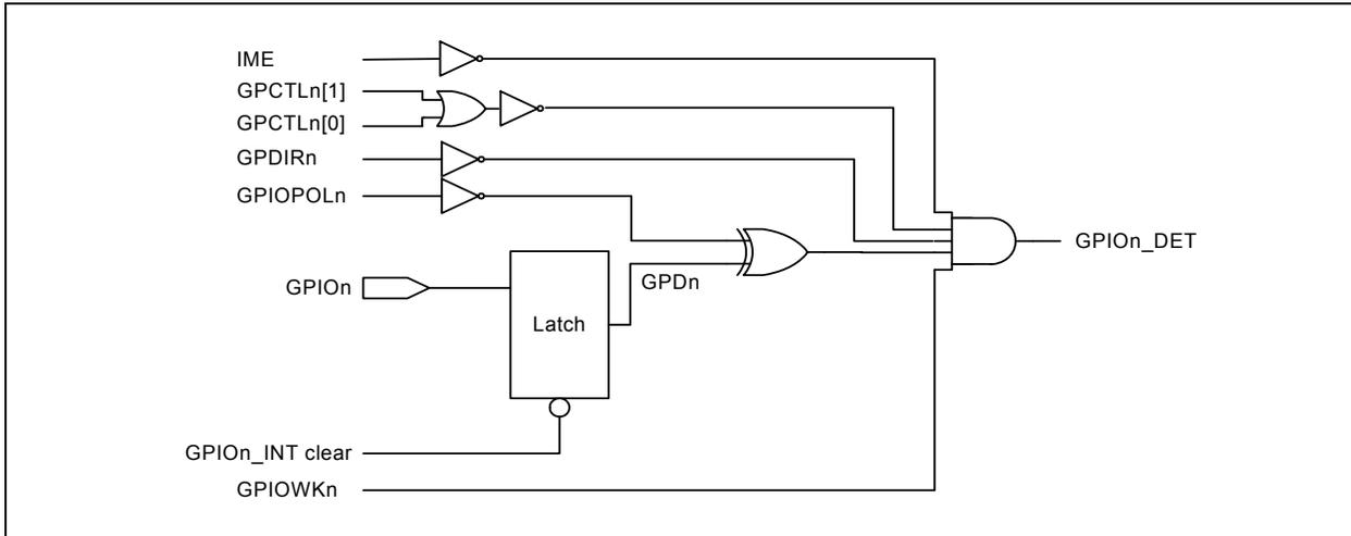
**Note:** The IME bit is in the [Hardware Configuration Register \(HW\\_CFG\)](#). [LED General Purpose IO Configuration Register \(LED\\_GPIO\\_CFG\)](#) and [General Purpose IO Wake Enable and Polarity Register \(GPIO\\_WAKE\)](#) must be set accordingly. Diagram does not represent actual hardware implementation.
