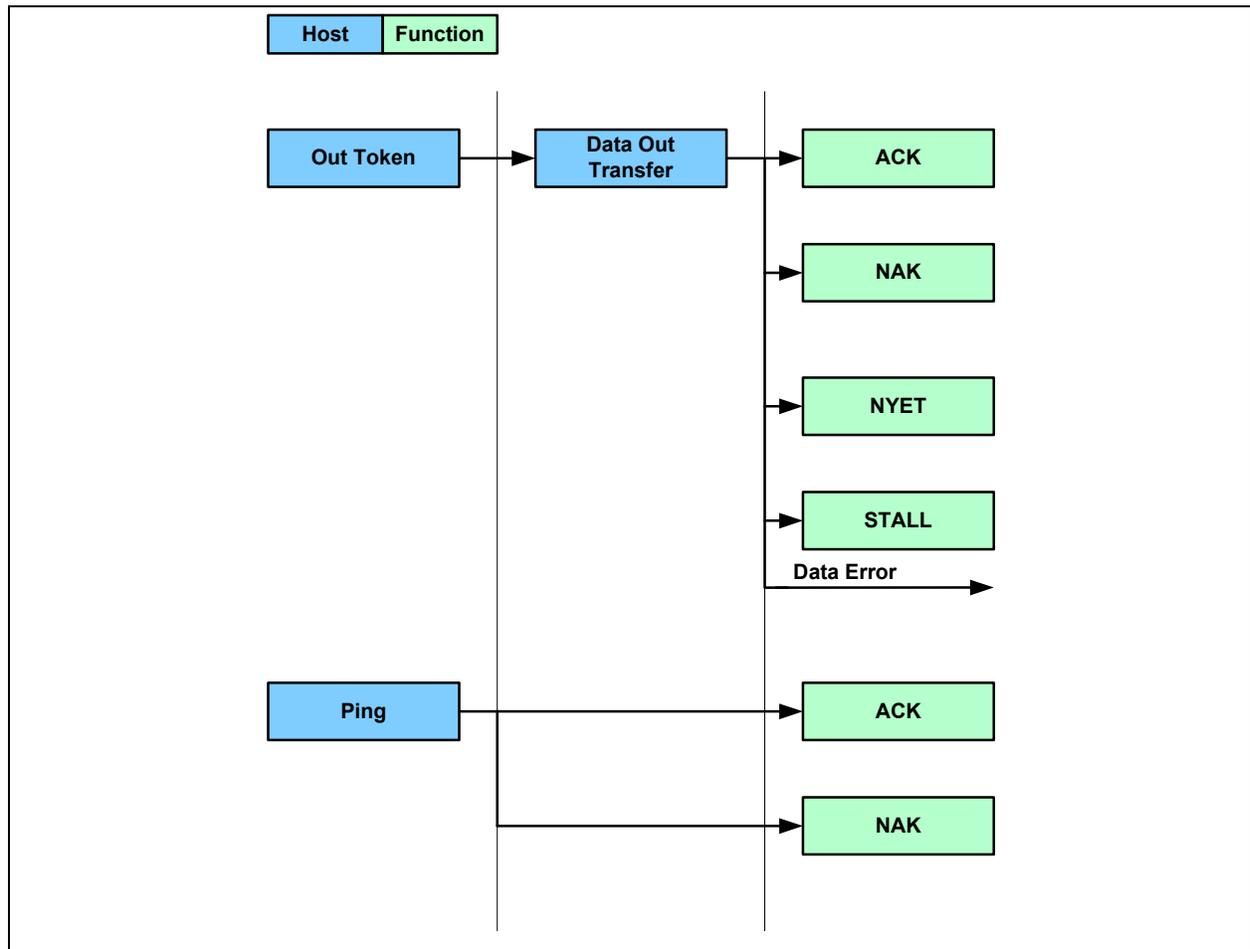
In the case where the Bulk-Out packet is errored, the URX does not respond to the host. The URX will request that the FCT rewinds the packet. It is the host's responsibility to retransmit the packet at a later time.
