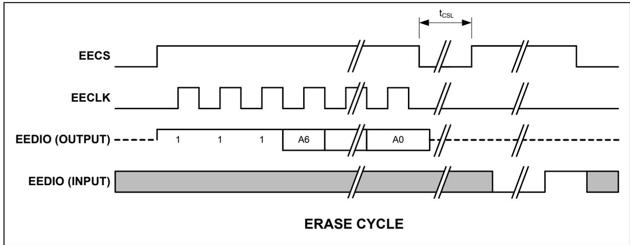
**ERAL (Erase All):** If erase/write operations are enabled in the EEPROM, this command will initiate a bulk erase of the entire EEPROM. The EPC\_TO bit is set if the EEPROM does not respond within 30 ms.
