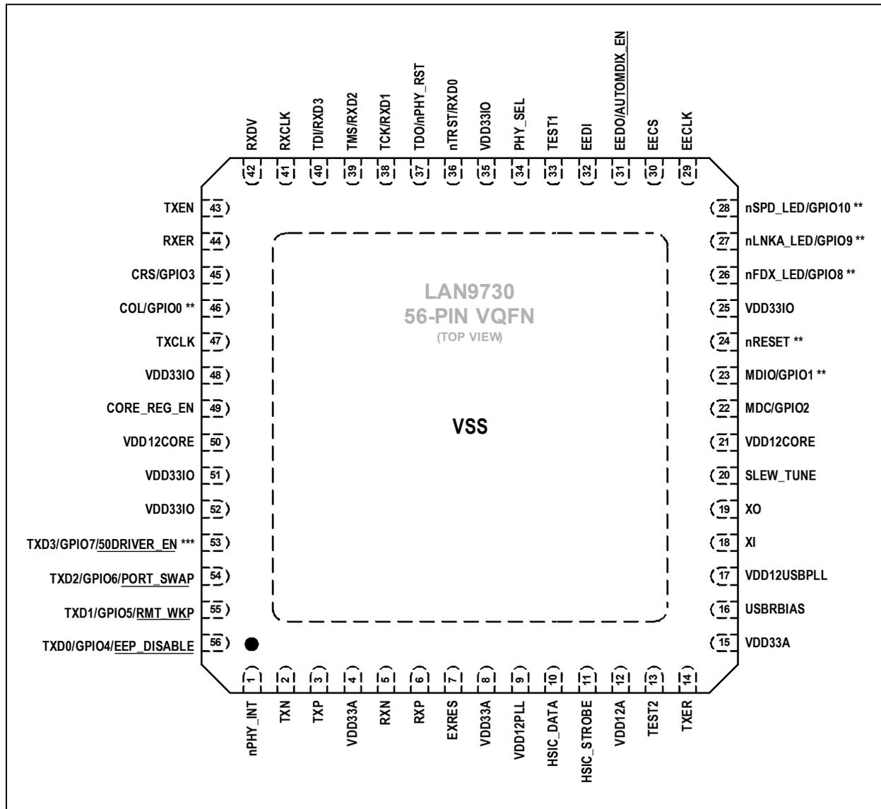
**Note:** \*\* This pin provides additional PME related functionality. Refer to the respective pin descriptions and [Chapter 5.0, "PME Operation"](#) for additional information.
