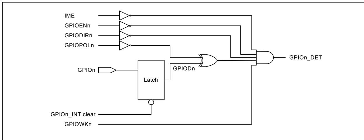
**Note:** The IME bit is in the [Hardware Configuration Register \(HW\\_CFG\)](#). [General Purpose IO Configuration Register \(GPIO\\_CFG\)](#) and [General Purpose IO Wake Enable and Polarity Register \(GPIO\\_WAKE\)](#) must be set accordingly. Diagram does not represent actual hardware implementation.
