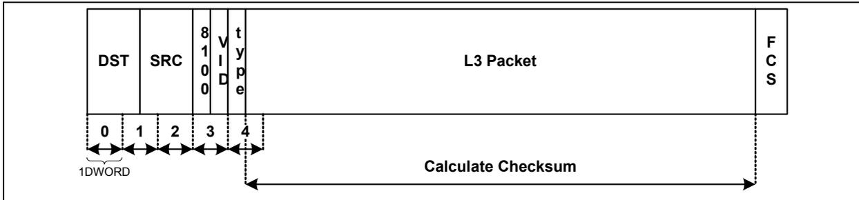
**FIGURE 4-13: ETHERNET FRAME WITH LENGTH FIELD AND SNAP HEADER**
