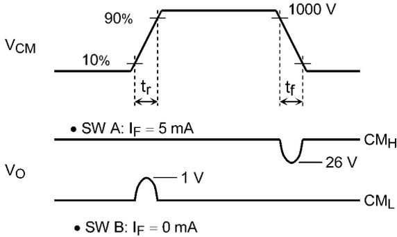
Fig. 13.1.8 Common-Mode Transient Immunity Test Circuit and Waveform
