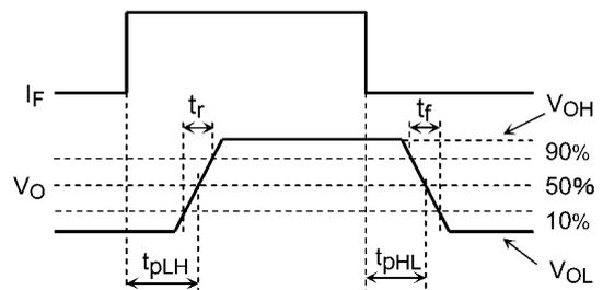
Fig. 13.1.7 Switching Time Test Circuit and Waveform
