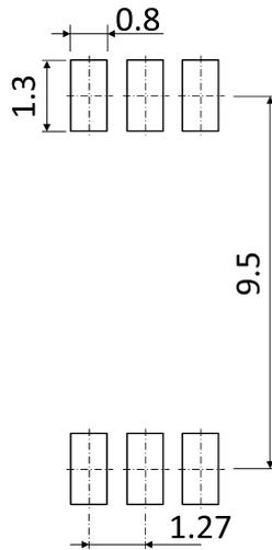
Fig. 15.1 Lead Forming Option (standard)
