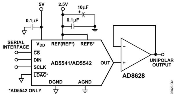
Figure 66. AD8628 Used as an Output Amplifier
