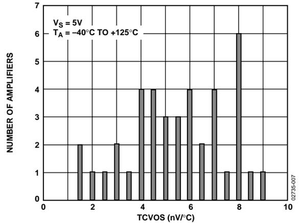
Figure 11. Input Offset Voltage Drift
