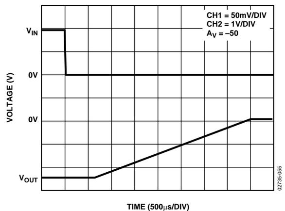
Figure 60. Positive Input Overload Recovery for LMC2001
