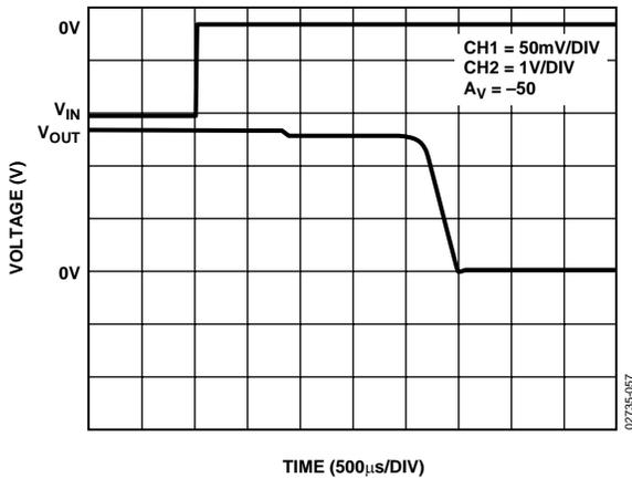
Figure 62. Negative Input Overload Recovery for LTC2050
