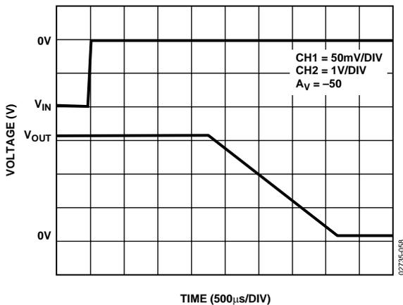
Figure 63. Negative Input Overload Recovery for LMC2001
