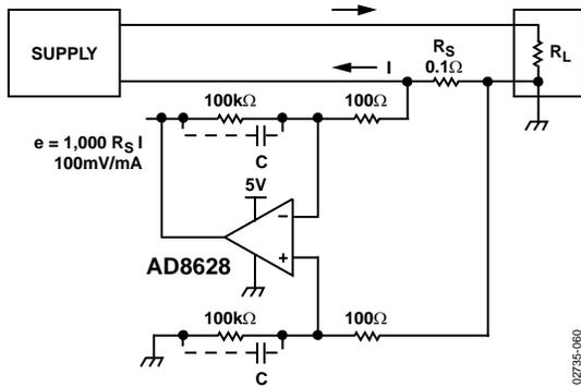
Figure 65. Low-Side Current Sensing
