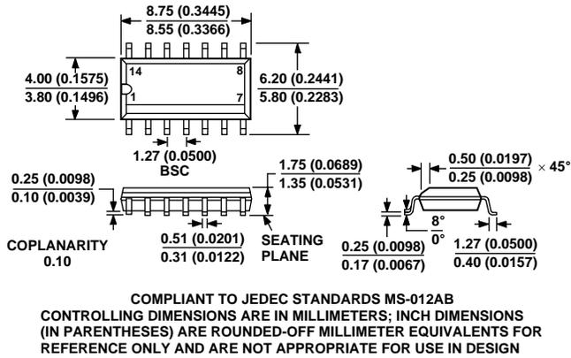
Figure 71. 14-Lead Standard Small Outline Package [SOIC]
