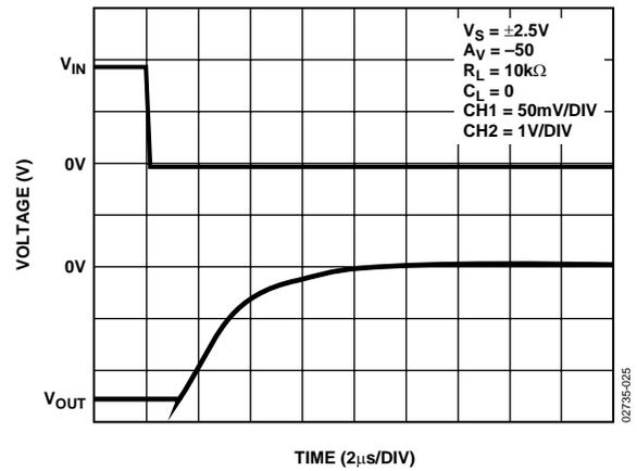
Figure 29. Positive Overtolerance Recovery
