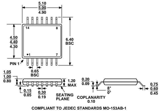
Figure 72. 14-Lead Thin Shrink Small Outline Package [TSSOP]
