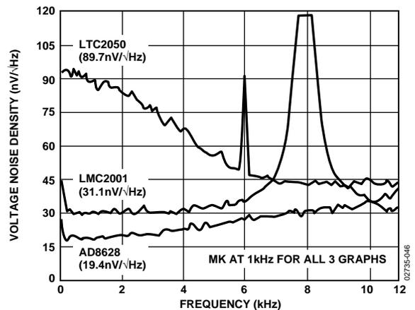
Figure 51. Noise Spectral Density of AD8628 vs. Competition
