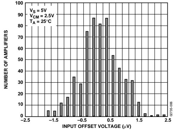
Figure 10. Input Offset Voltage Distribution at 5 V
