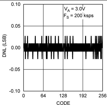
Figure 5. DNL –  $V_A = 3 \text{ V}$
