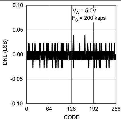
Figure 7. DNL –  $V_A = 5 \text{ V}$
