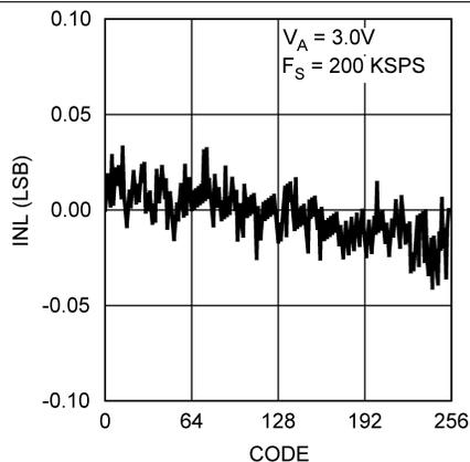
Figure 6. INL –  $V_A = 3 \text{ V}$
