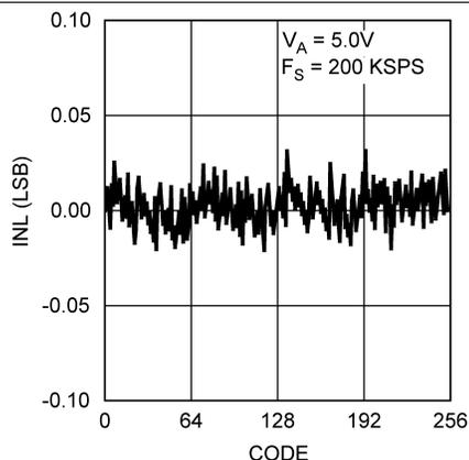
Figure 8. INL –  $V_A = 5 \text{ V}$
