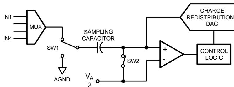
**Figure 47. ADC084S021 in Track Mode**
