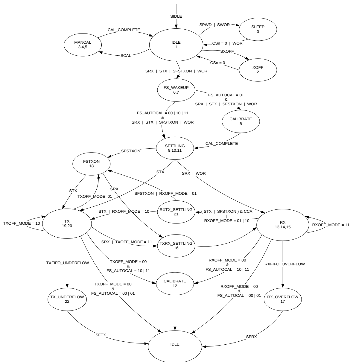
Figure 25: Complete Radio Control State Diagram
