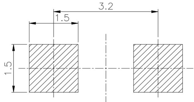
**Notes:** Tolerances Unless Dimension  $\pm 0.1\text{mm}$ , Unit = mm
