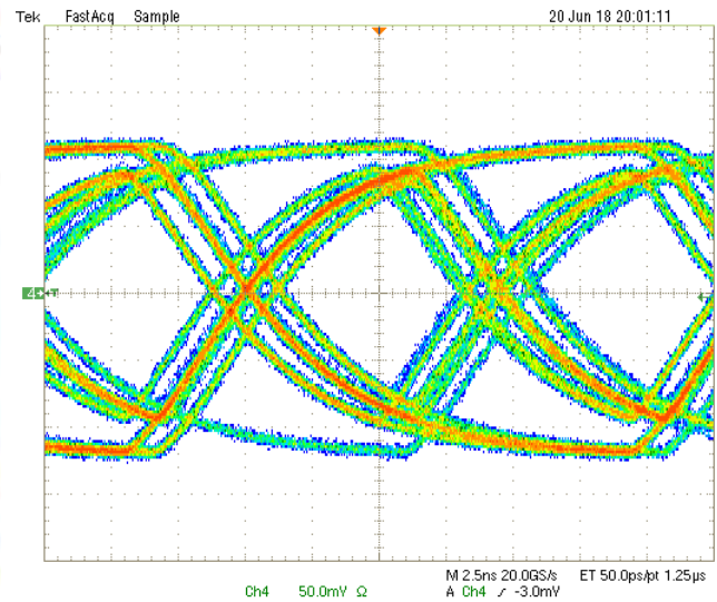
Figure 6-12. Back Channel Output Typical Waveform
