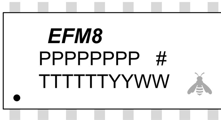
**Figure 9.3. SOIC16 Package Marking**
