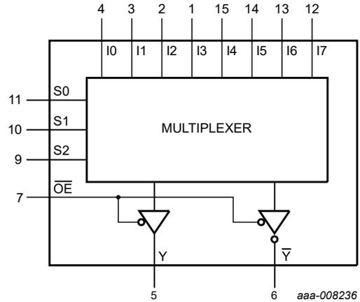
Fig. 2. Functional diagram
