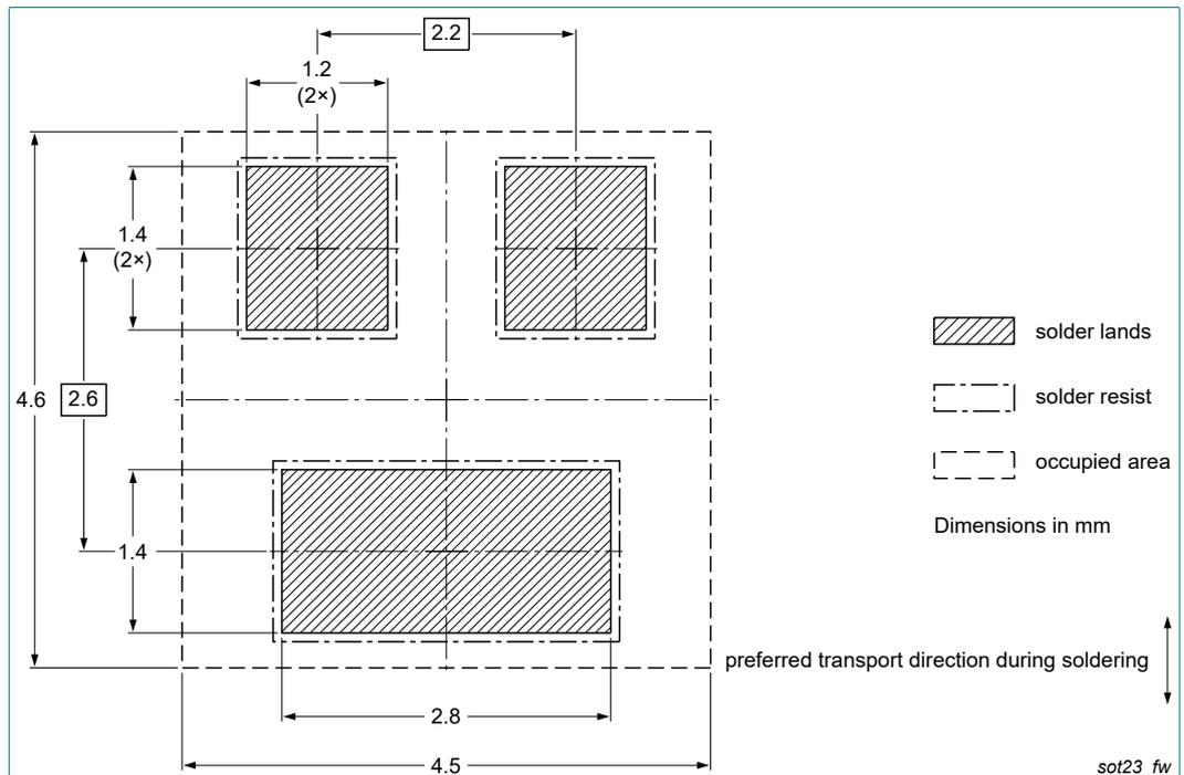
**Fig. 13. Wave soldering footprint for SOT23 (TO-236AB)**
