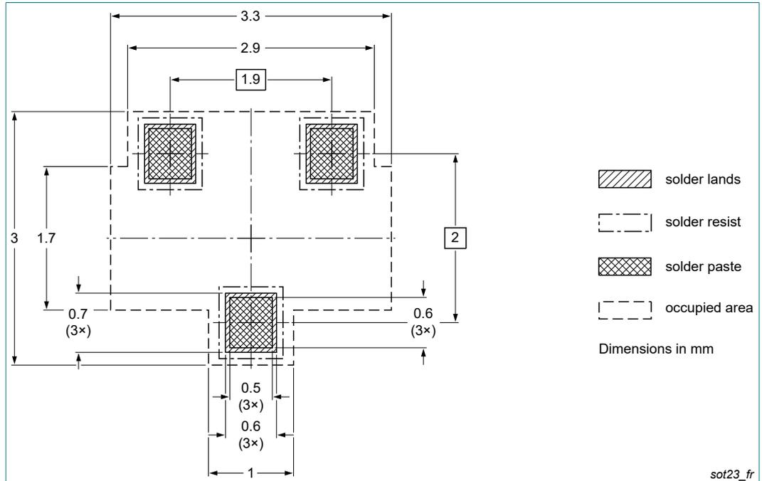
**Fig. 12. Reflow soldering footprint for SOT23 (TO-236AB)**
