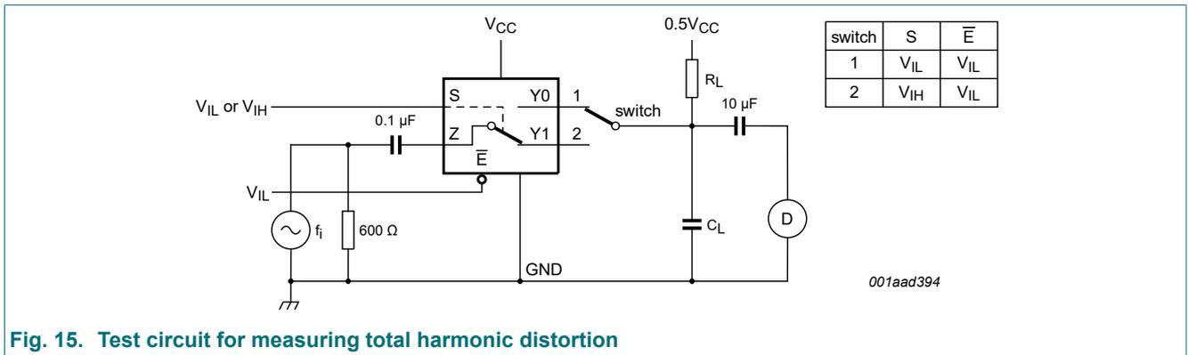
**Fig. 15. Test circuit for measuring total harmonic distortion**
